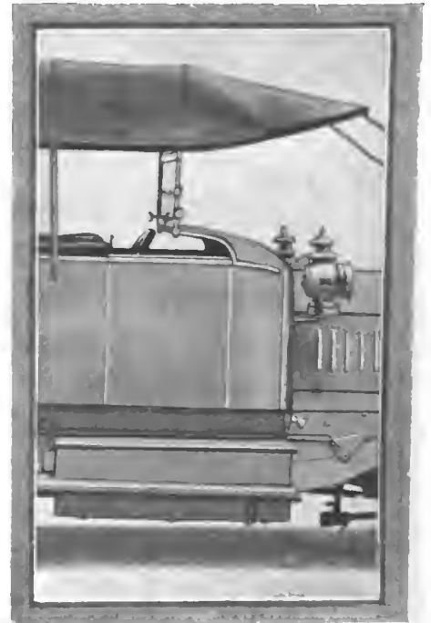
Fig. 9—Cowl extended so as to bring the windshield closer to the driver and the top given an extra extension for better protection
